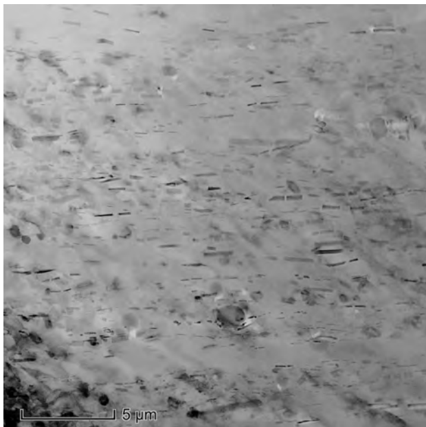
5E61 aluminum alloy: Al-6Mg-0.9Mn-0.07Zr-0.2Er (wt.%)
