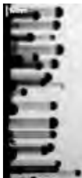
Nanowires grown in situ, characterized post-growth (F. Ross, IBM)
