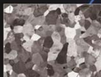
Sample: Pure Titanium Accelerating Voltage: 5 kV Magnification: 800x
